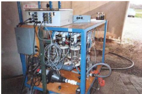
The Carew patented wave-coil centrifugal filter (WCF) and solids drying system along with its developing gasification/fuel cell technologies, when use alone or in combination with select complementary technologies, have the capability in the field to process municipal, agricultural, marine waste water, and most solid waste streams.
